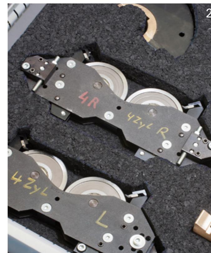
Fig.: 1 Optimized changeover concept with exchange fingers and shell inserts.
