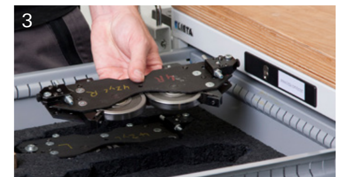
Fig.: 1 Optimized changeover concept with exchange fingers and shell inserts.
