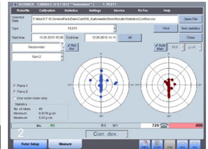
Fig.: 1, 2 CAB 950 – the measuring instrument for series production - simple operation, highly accurate measured value recording, precise correction calculations.
